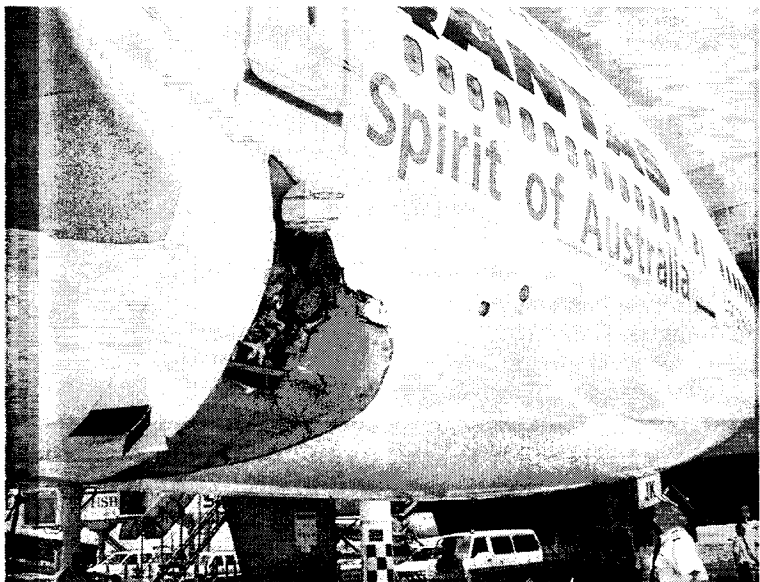
Manila, 25 July 2008: Qantas pilot inspects damage after oxygen tank exploded mid-flight. Airline attacks on unions compromise safety.
